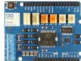
Arduino Motor Shield
